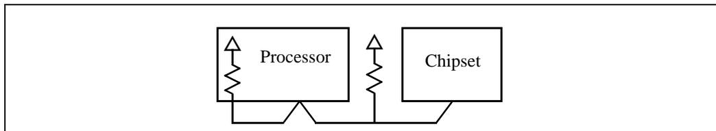
**Figure 3. AGTL+/AGTL Bus Topology in a Dual-Processor Configuration**
