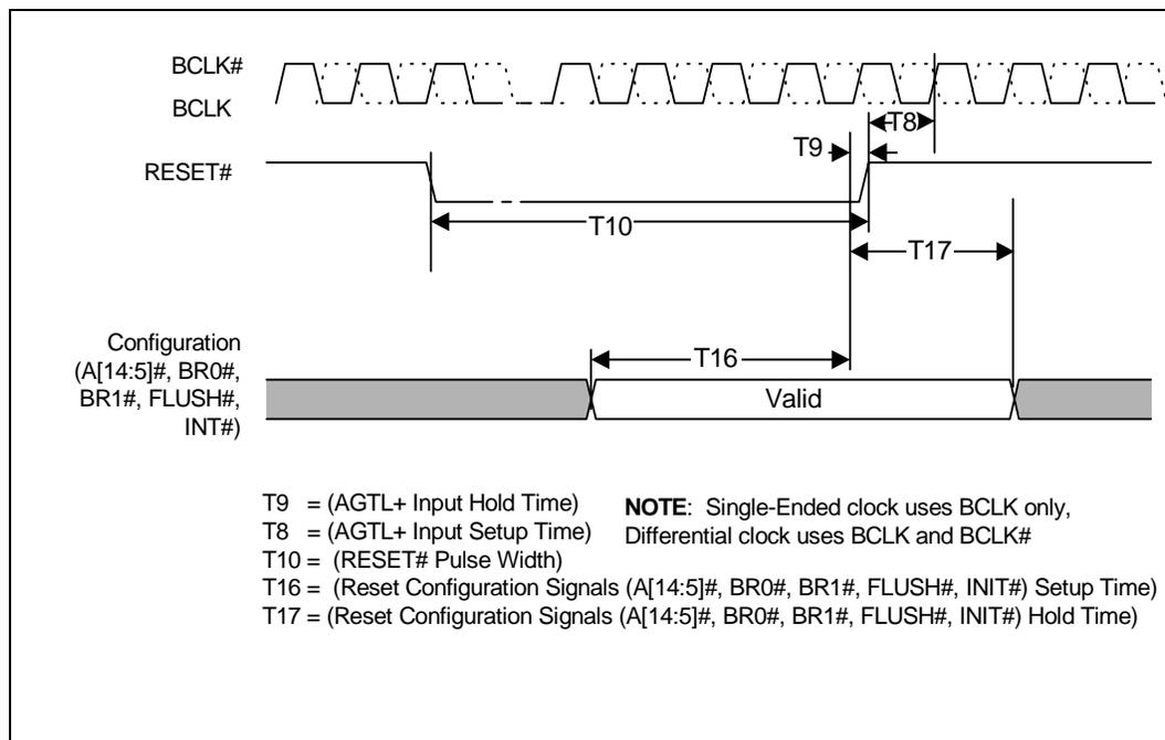
Figure 14. Platform Power-On Sequence Timings
