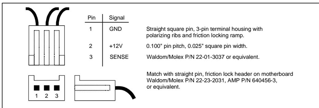
**Table 41. Fan Heatsink Power and Signal Specifications**
