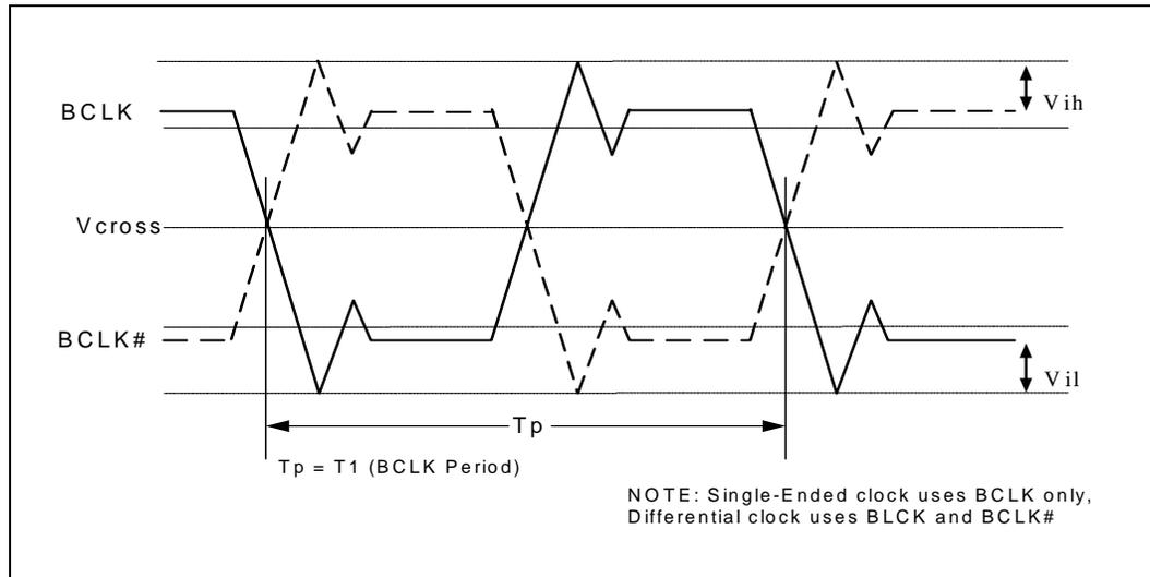
Figure 10. BCLK, PICCLK, and TCK Generic Clock Waveform
