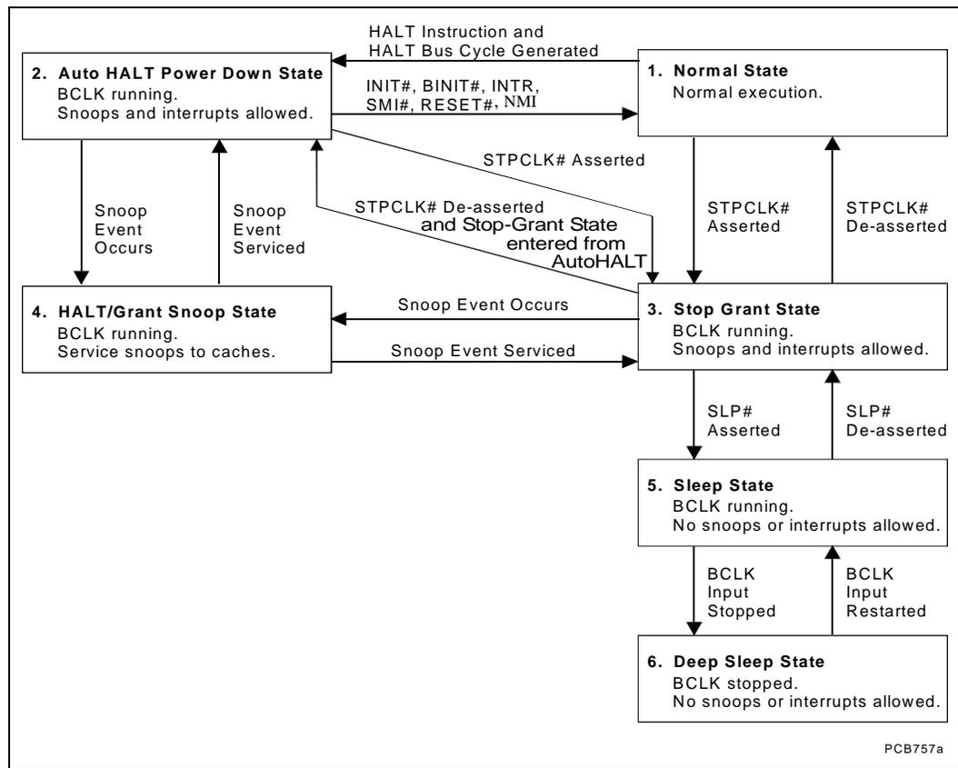
For the processor to fully realize the low current consumption of the Stop-Grant, Sleep and Deep Sleep states, a Model Specific Register (MSR) bit must be set. For the MSR at 02AH (Hex), bit 26 must be set to a '1' (this is the power on default setting) for the processor to stop all internal clocks during these modes. For more information, see the *Intel Architecture Software Developer's Manual, Volume 3: System Programming Guide* located on the developer.intel.com website.
