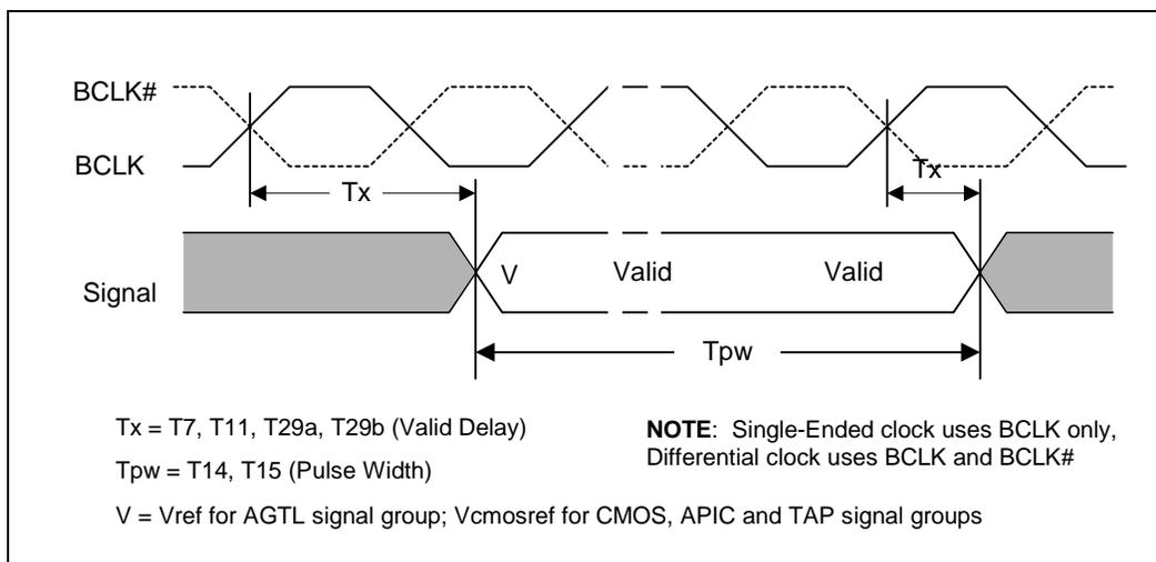
Figure 12. System Bus Setup and Hold Timings
