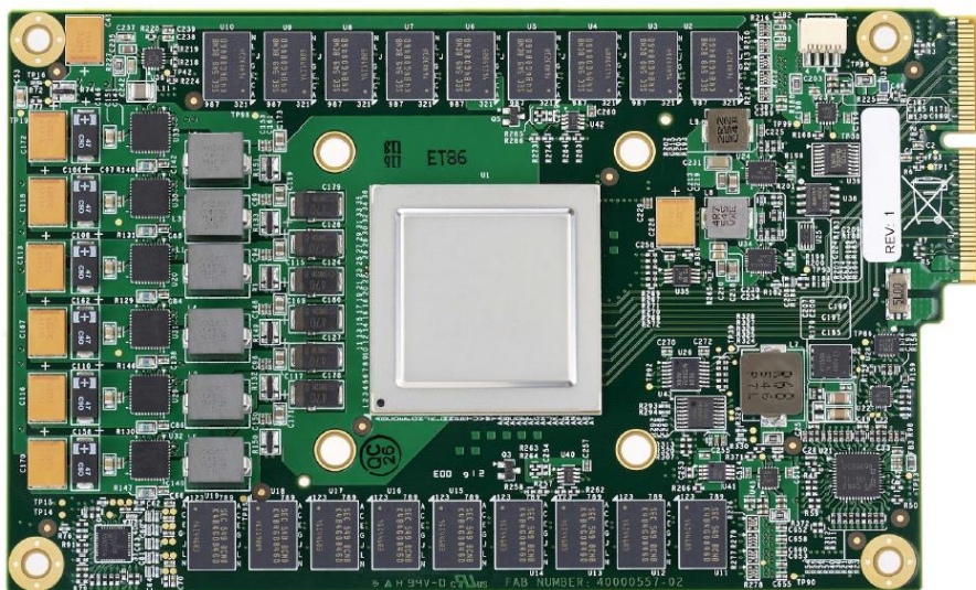
Figure 3. TPU Printed Circuit Board. It can be inserted in the slot for an SATA disk in a server, but the card uses PCIe Gen3 x16.
